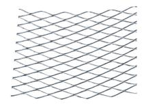
Quality: Manufactured from galvanised steel to BS EN 10346: 2009 – DX51D+Z275 or Stainless Steel to BS EN 10088-2-1.4301. All products shown are manufactured in accordance with BS EN 13658: 2005. Metal Lath - Definitions, Requirements, Test Methods. Part 1 for Internal Plastering. Part 2 for External Plastering.
